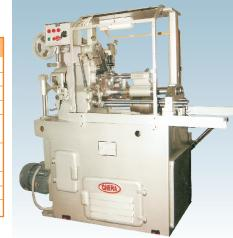
**Standard accessories**: Cross Slide, Tail-Stock with collet mechanism, Bar Feed Attachment, Electrical equipments with control panel, Motors, Coolant Pump with fittings, Set of change gears, Set of hand tools, Splash guards, Chip tray, Weights, Pusher rod, Rope for bar feed, Grease Gun, Stand.
